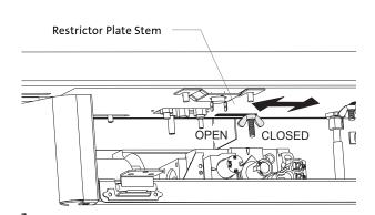
Figure 28. Air Inlet Restriction Adjustment
